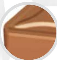
Optimised geometry for negative inserts giving perfect chip control at a wide range of cutting data. Mainly applied for finishing and semi-finishing machining of steels and stainless steel materials. The precision grinding techniques gives high dimension accuracy and high indexing repeatability. Specially designed rake face structure ensures insert strength while greatly reducing the cutting forces. Advanced edge preparation and new coating for excellent surface finish.
