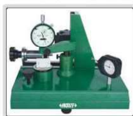
Test repeatability of dial indicators
