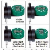
Remark: To change above direction, 4 fixing screws on the back of display need to be removed first.
