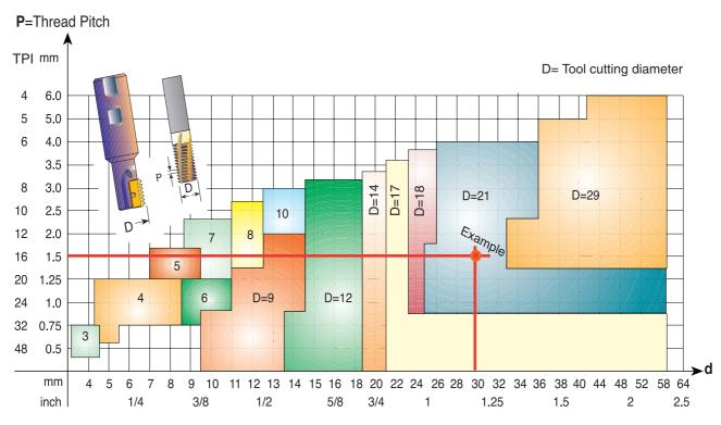
Any tool with a small cutting diameter can produce large diameter threads.
