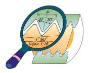
Conical pipe thread inserts are onesided and may be used for both External and Internal threading.
