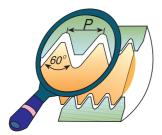
Same Insert for External and Internal thread
