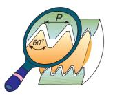
Same Insert for External and Internal thread
